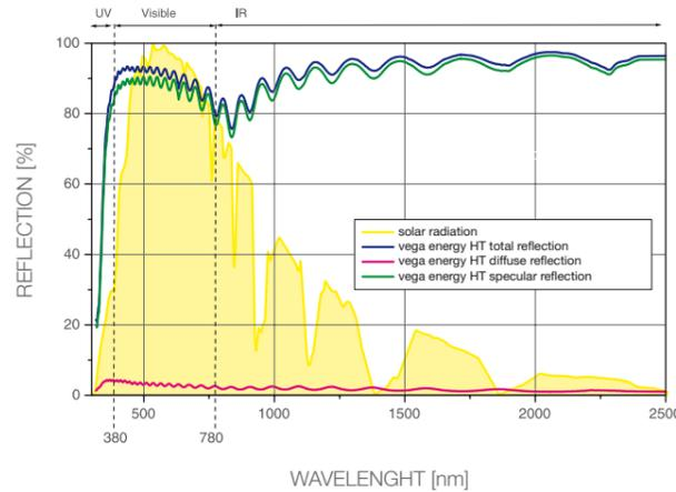
Designed to maintain constant high levels of reflection even at continuous operating temperatures of up to 250 C, **vega energy HT** is the ideal surface to be used in the secondary reflectors of the Fresnel systems. Its special coating greatly reduces the degradation phenomena of the reflecting surface, ensuring high performance over the long run.
